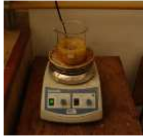
Fig. 5 – Device used in flotation using NaOH as heavy liquid experimental tests.
